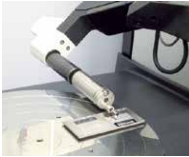
Measurement example) R axis direct operated roughness measurement (roughness specimen)
